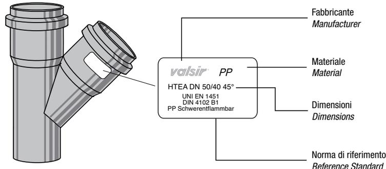
*The Valsir PP system is characterised by push-fit connections with seals and consequently does not require expansion sockets, in that each joint, when correctly installed, allows the material to expand and contract in the presence of temperature fluctuations.*
